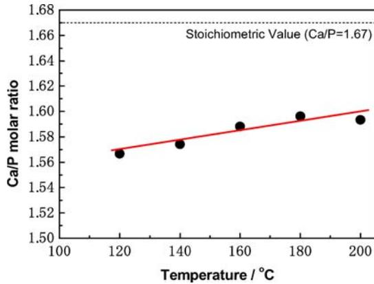
Figure 2 Ca/P molar ratio of rod-shaped HA particles prepared by hydrothermal vapor exposure method at the indicated particles temperature for 5 h.
