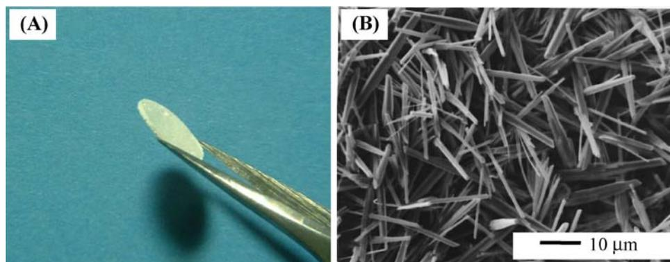
Figure 1 Sheet of HA prepared by hydrothermal method at 120°C under saturated vapor pressure for 3 h (A). Rod shaped crystals were observed by SEM (B).
