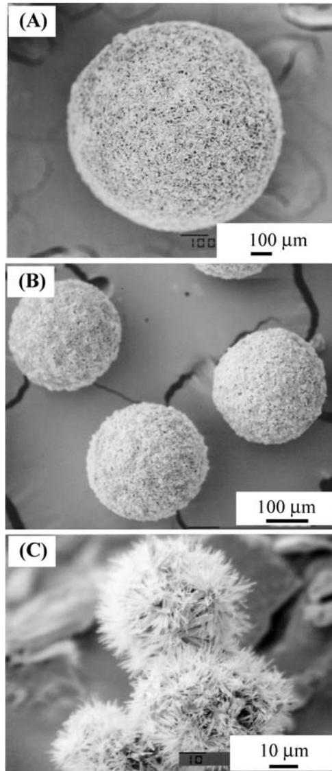
Figure 3 Scanning electron micrographs of HA granules prepared by hydrothermal vapor exposure method at 160°C for 3 h. The stirring rate was (A) 0 r.p.m., (B) 300 r.p.m. and (C) 900 r.p.m.
