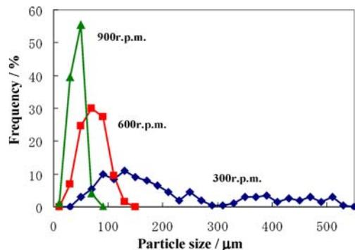
Figure 4 Particle size distribution of HA granules prepared at the indicated stirring rate.
