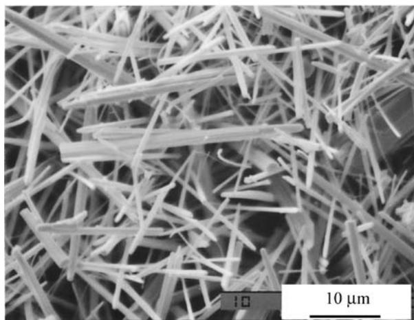
Figure 5 Scanning electron micrograph of the HA granule (Fig. 3(A)) prepared by hydrothermal vapor exposure method.
